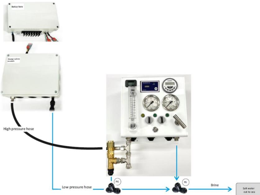
The picture below shows an overview of how the product's parts should be placed in the system with the "Flush" control panel for connecting the high-pressure and low-pressure hoses
