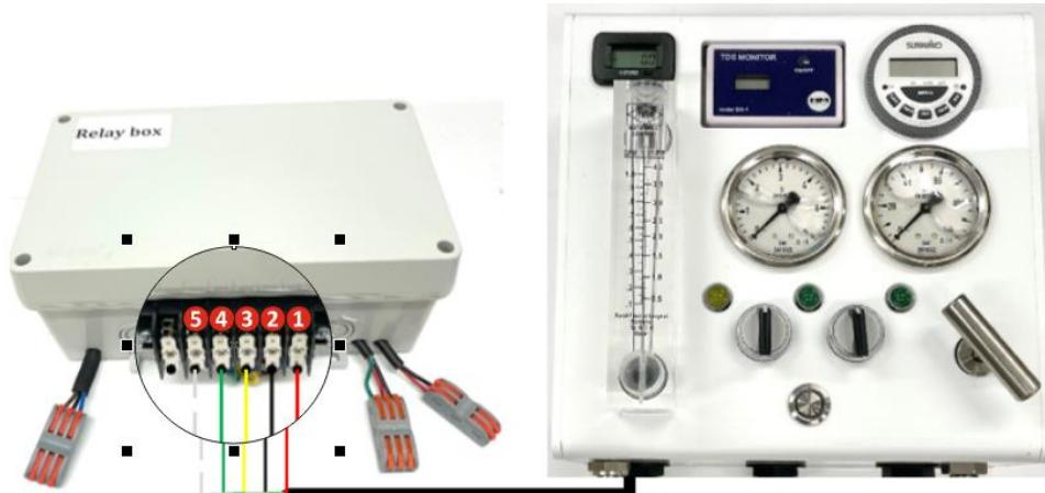
4 Connect the boost pump (seawater pump) with the cooling fan to the terminal block + (4 green) and – (2 black).
